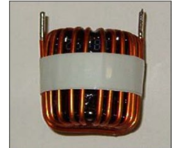
Leads are wire of coil & secured with tape to body of coil for thru-hole mounting to circuit board.
