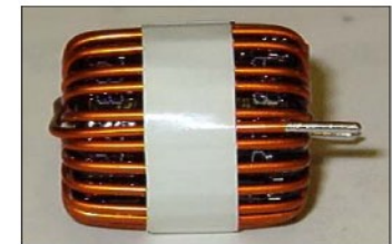
Finished coil is dipped in air dry varnish.
