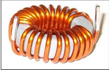
Part number: 140-0005 Toroidal power inductor.
