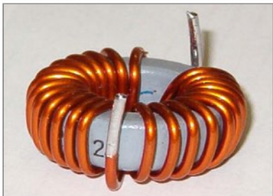
Leads are wire of coil which are stripped & tinned to mount on thru-hole circuit board.
