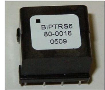
Part number: 80-0016 Core encloses coil providing shielding from outside interference. Cores are presently cemented together.
